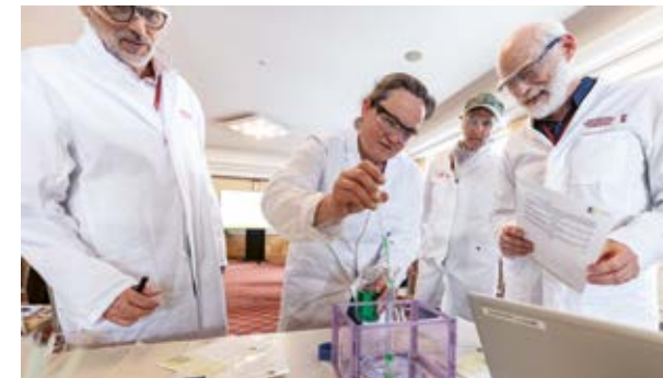
Measuring the film thickness of a soap bubble
